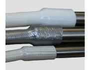
**GVES4000EXP** is an insulating sleeving made of braided fiberglass yarn coated with silicon resin. The special braiding and the special coating allows the diameter to expand up to 60% from original diameter and it is generally softer in comparison to standard GVES. It is recommended for sleeving applications that require a snug fit over irregular shapes.
